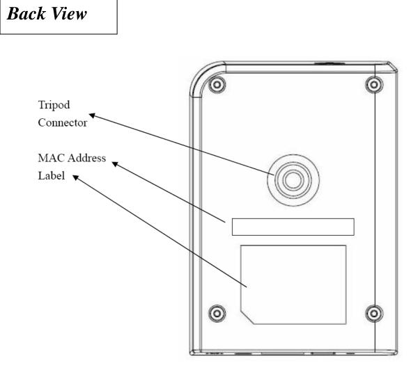
Tripod Connector: Connects to any standard tripod / camera wall holder. MAC Address Label: Shows the MAC address of this Network Camera. Useful when you can't locate the camera on the network.
