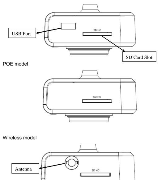
SD Card Slot: Accepts SD / SD-HC memory card for image / video storage USB Port: Connects to certain wireless module. Antenna Base: Connects to supplied antenna
